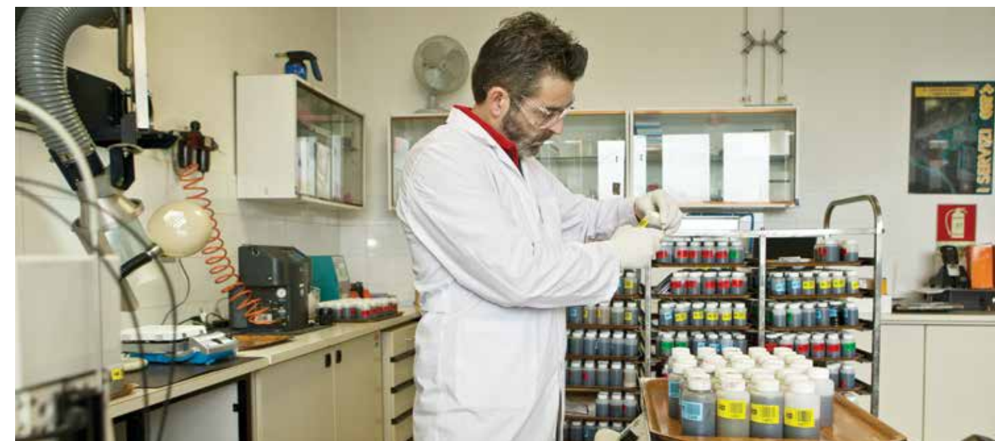
Once the oil sample is collected, it is sent to a lab for analysis. The lab looks for indicators of wear, contamination, and other issues that may be affecting the performance of the machine.
